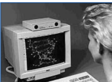
Figure 6 - The HeadMouse wireless optical sensor unit sits on top of the monitor.
